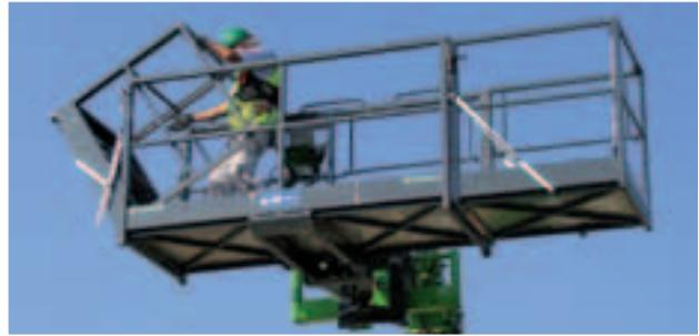
▶ Several Merlo platforms have a **hydraulic slewing function**, thus making it possible to work whatever the machine's position.
