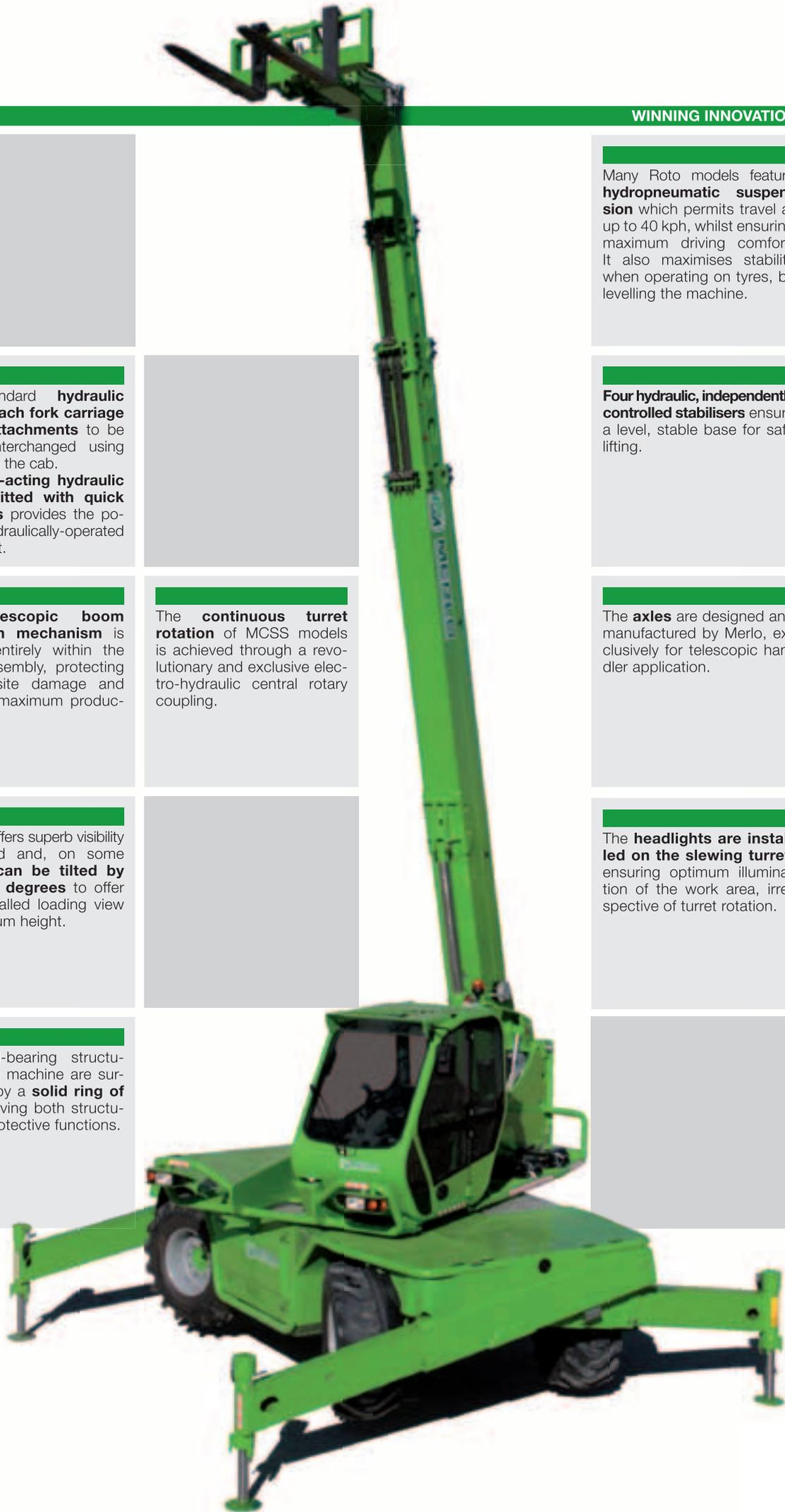
The standard **hydraulic quick-attach fork carriage** allows attachments to be quickly interchanged using controls in the cab. A **double-acting hydraulic service fitted with quick couplings** provides the power for hydraulically-operated equipment.
