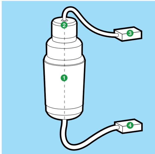
▶ The **central rotary electro-hydraulic joint** includes a separate stainless steel section, which circulates hot water generated by the diesel engine to heat the cab. There is, therefore, no need to install an auxiliary cab heating system.
