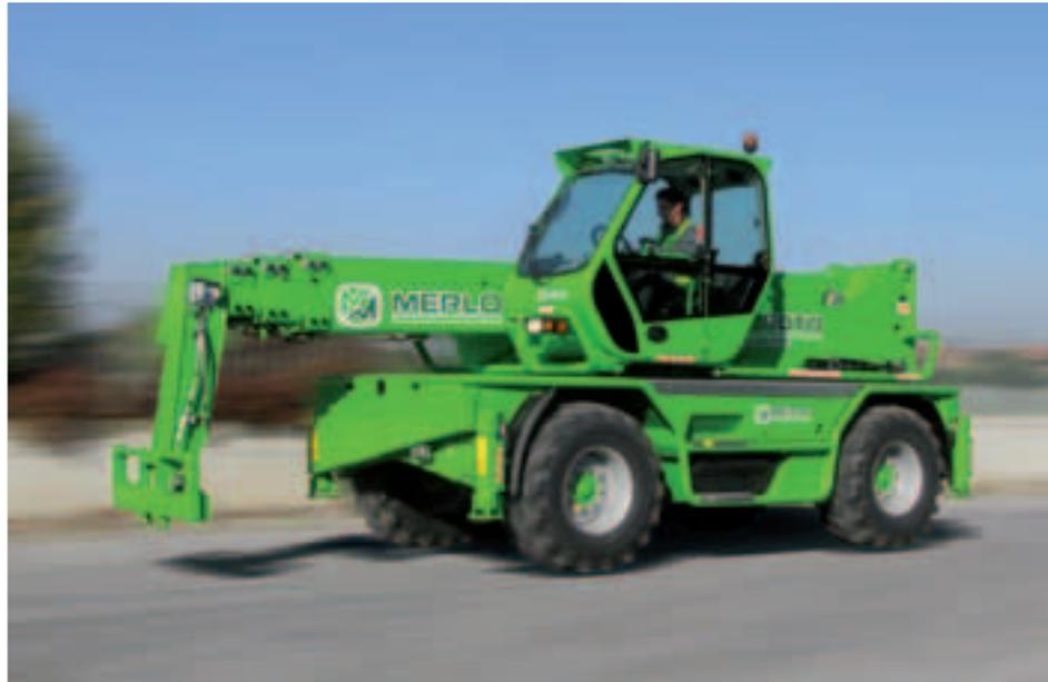
◀ The suspension can be locked in any desired position, so as to ensure the necessary **stability and safety** during any lifting operations whilst the machine is used 'on-tyres'.
