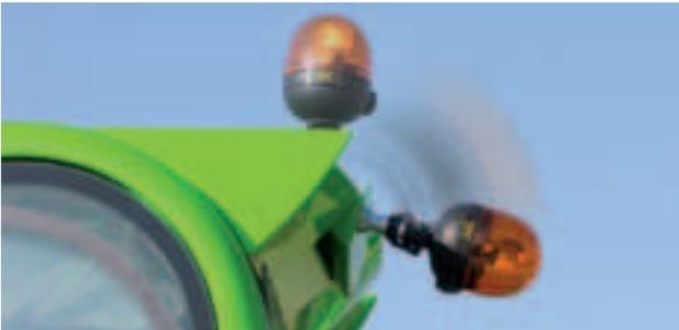
◀ The **rotating beacon folds down** to reduce overall height.
