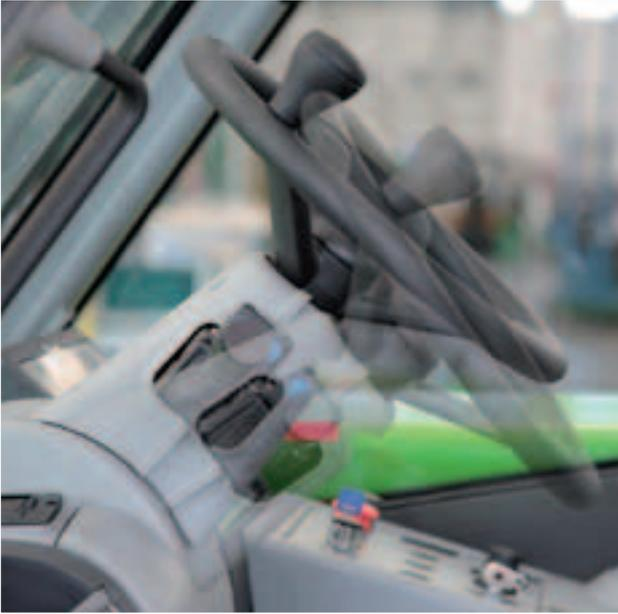
◀ The **steering wheel tilt** can be adjusted by up to 16 degrees, to match diverse driver shapes and sizes.
