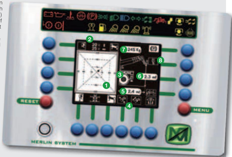
1 - Position of the centre of gravity relative to the working area; 2 - Longitudinal and transversal stability indicator; 3 - Stability status of the machine; 4 - Limitation of working area; 5 - Distance between the load and the turret centreline; 6 - Distance between the load and the ground; 7 - Weight of the load being handled; 8 - Equipment type in use.
