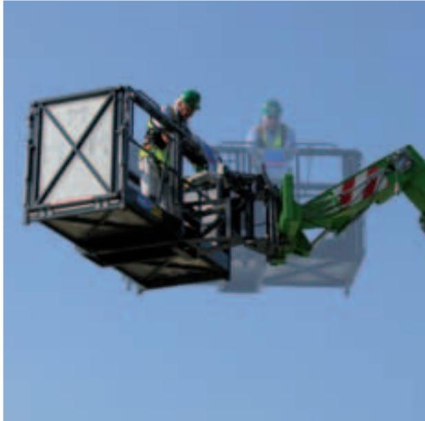
▲ The useful width of this Merlo platform attachment can be adjusted with the **patented extension system**, even whilst elevated!
